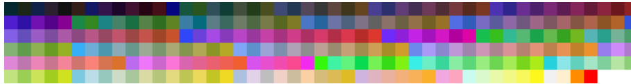
Fig. 2. Palette of M = 279 colors obtained by sampling the CIELAB color space on a body centered cubic lattice. The two last orange and red colors have been added manually.
